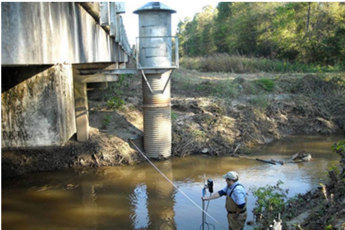
Figure 9: Stream flow measurement at station 15260 in Segment 0405A
