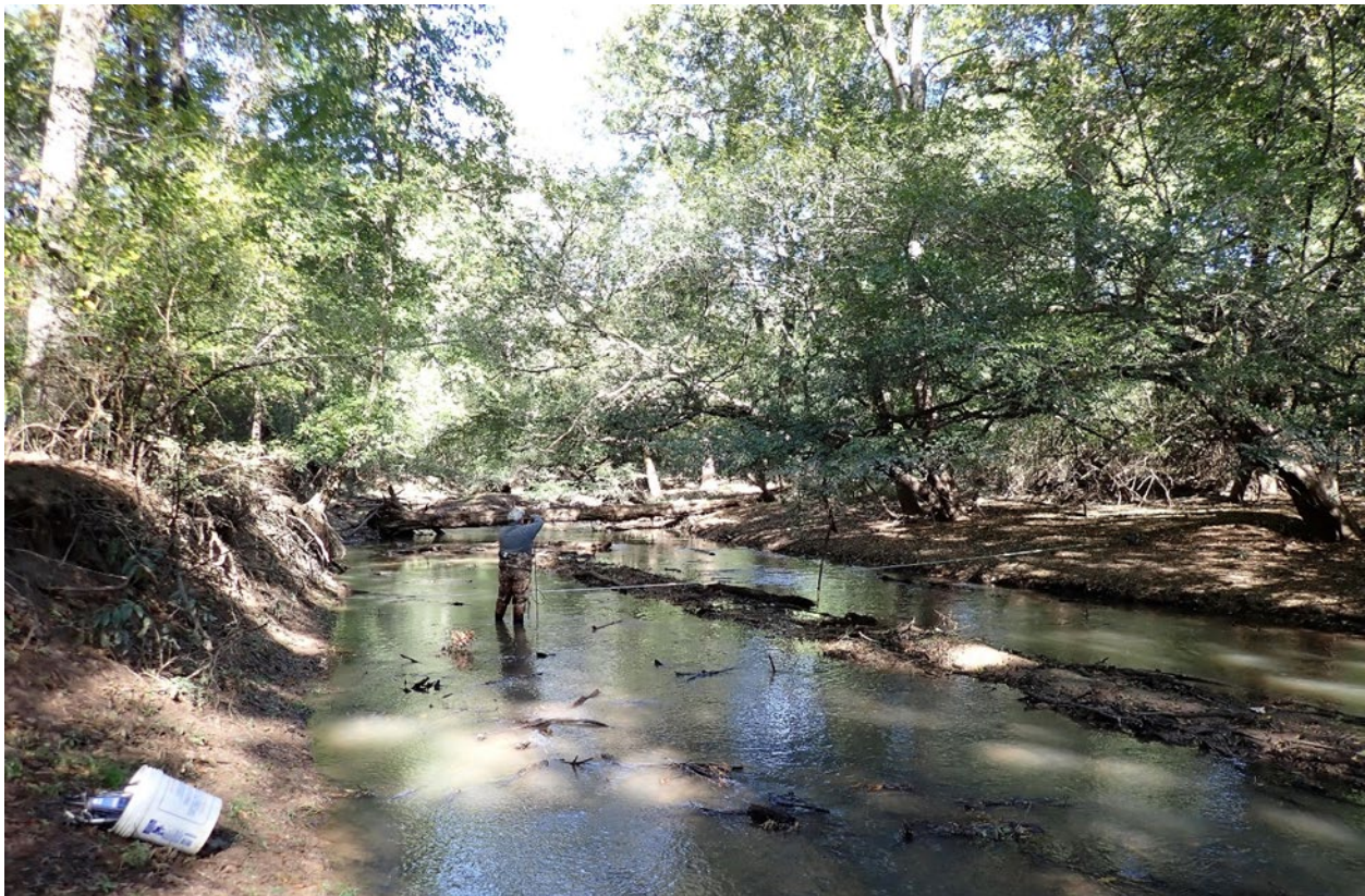
Figure 15: Stream flow measurement at station 16458 in Big Cypress Creek
