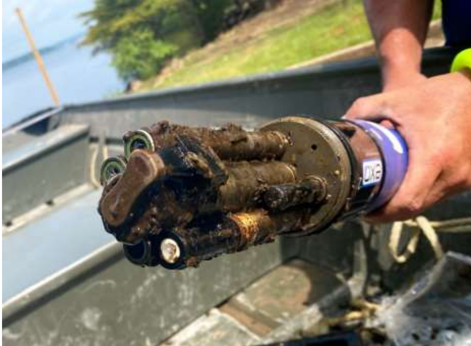
Figure 18: Water Quality Sonde After Eight-Week Deployment at NETMWD Intake
