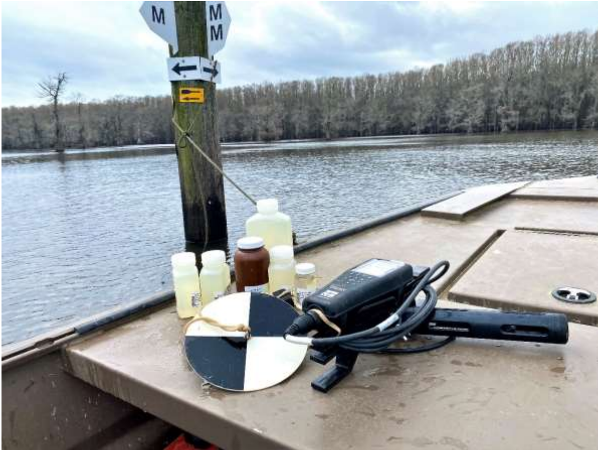
Figure 8: Sample bottles and instruments used to measure field parameters
