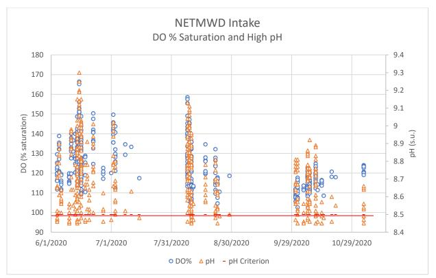
Figure 41: NETMWD Intake: DO percent saturation and High pH
