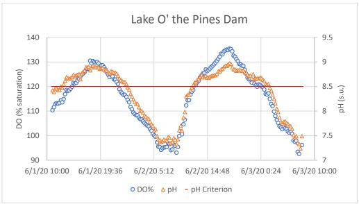
Figure 47: Lake O' the Pines Dam Station: DO percent saturation and pH
