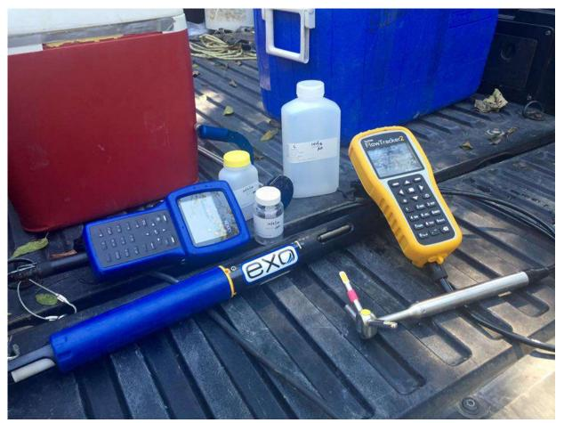
Figure 7: Sample bottles and instruments used to measure field parameters and stream flow
