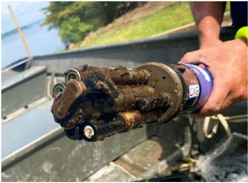
Figure 37: Water Quality Sonde After Eight-Week Deployment at NETMWD Intake
