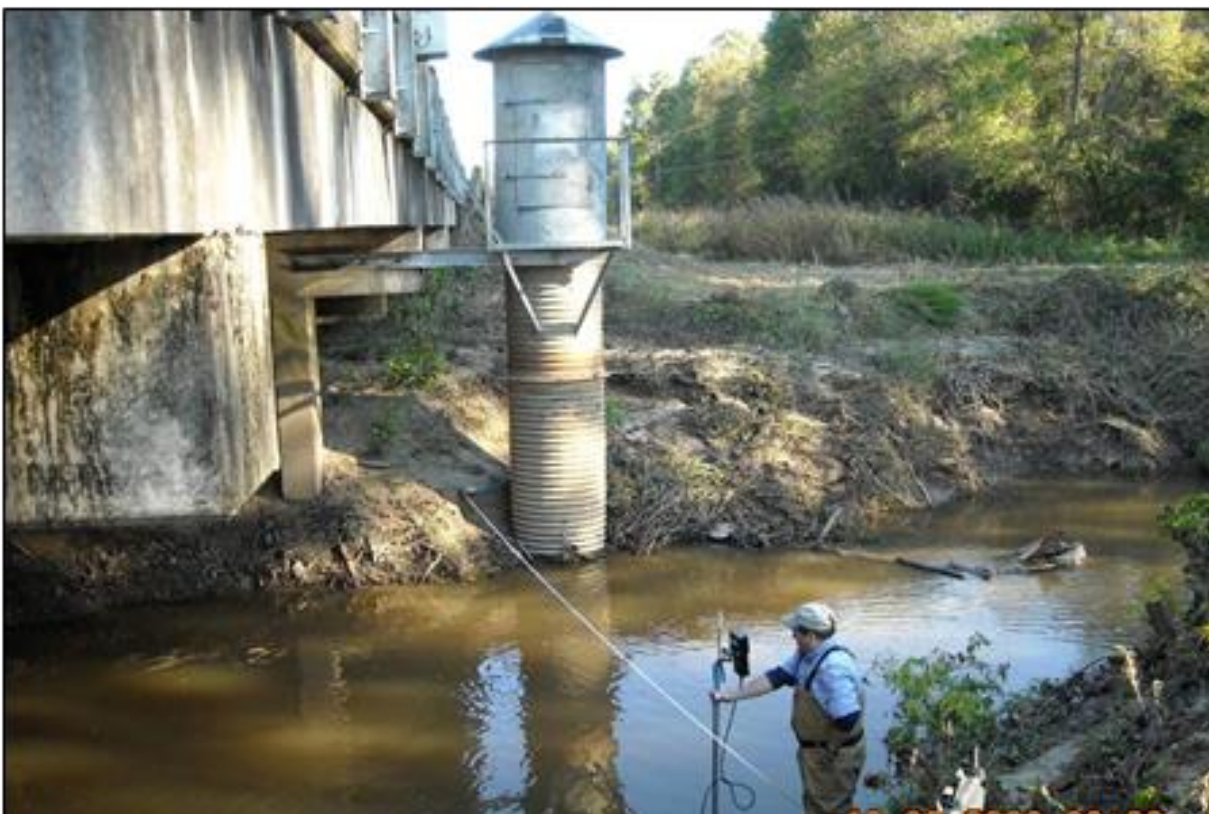
Figure 23: Stream flow measurement on Big Cypress Creek at SH 37
